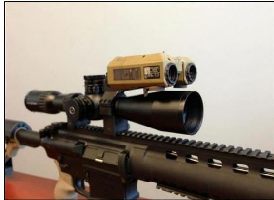
Figure 3. The RAPTAR mounted on top of a riflescope is a perfect example of a separation of the laser rangefinder optics from the direct-view optics.
